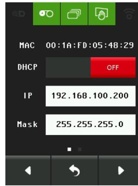
**Step 3:** Unplug the USB cable and install all the hardware equipment (please refer to diagrams in section Using a Switch). Make sure the printer is switched on and the Ethernet cables are plugged. Make sure to retrieve the IP address provided by the DHCP server to the printer. Then go to [Finishing the Printer Configuration](#) <sup>22</sup>.
