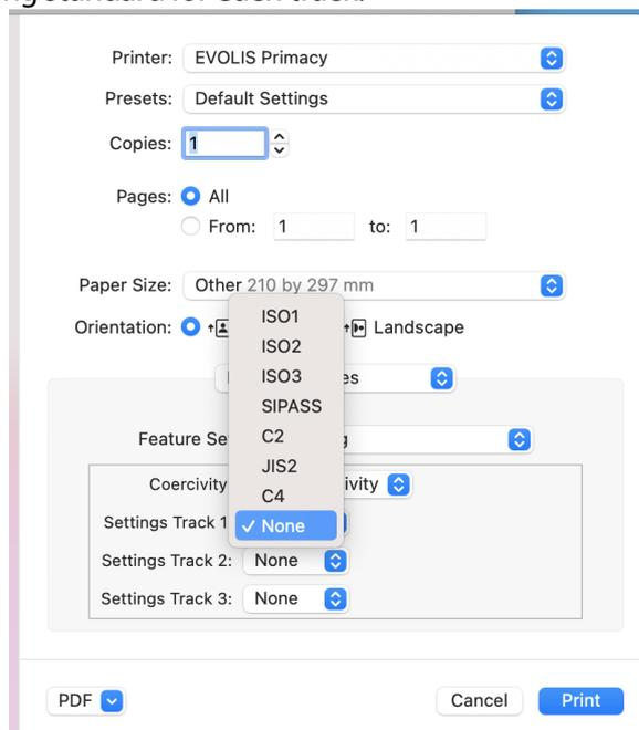
The stripes can be configured in ISO, SIPASS, C2, JIS2 and C4 format. See the tables below for information on the ISO 7811 and JIS2 (Japanese Industrial Standard) standards.
